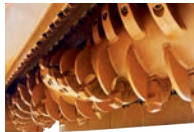
Rigid Tungsten-Carbide Tooth Rotor (Smooth cut)
